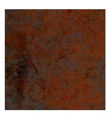
Thanks to the process of oxidation and maturation that characterizes it, The Corten Steel is considered a live material, which may vary over time, in shades and hues, depending on the shape of the object, the position in which it is installed and according to the cycles of weathering which the object undergoes.
